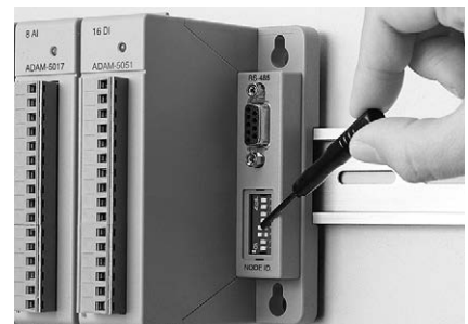
Node ID Setting 8-pin dip switch configuration
