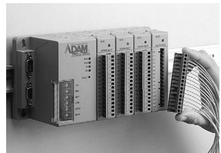
Connection Pre-wired plug-in terminals with I/O modules
