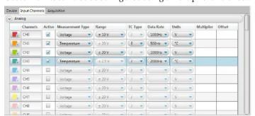
Activate the analog channels to include in the acquisition from the **Analog** section of the **Input Channels** tab. Channel options include measurement type, voltage range, TC type, data rate, and units.
